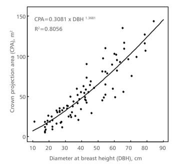
**FIGURE 4.** Relationship of the crown projection area (CPA) and the DBH
